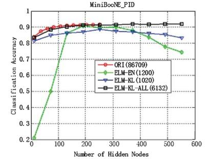
(b3) The curves of testing accuracy on dataset MiniBooNE
