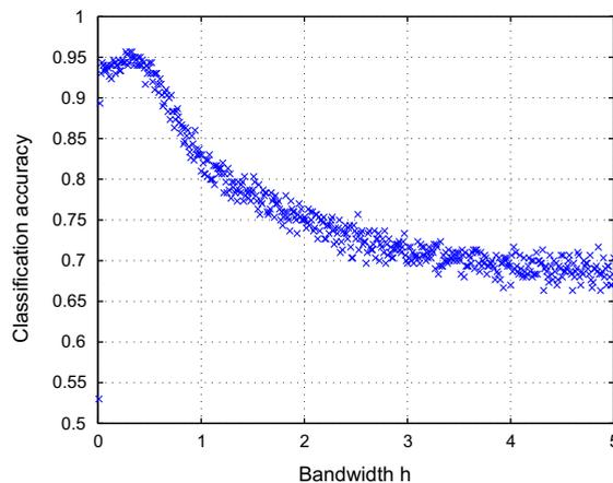
**Fig. 3.** The sensitivity of bandwidth on classification accuracy in single fault dataset SinglFG (100).
