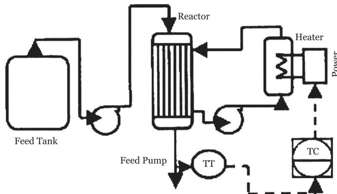
Fig. 9. The schematic diagram of chemical process [24,4].
