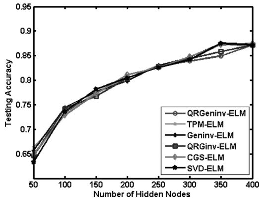
Fig. 3. The testing accuracy of the six algorithms in Letter with different number of hidden nodes.
