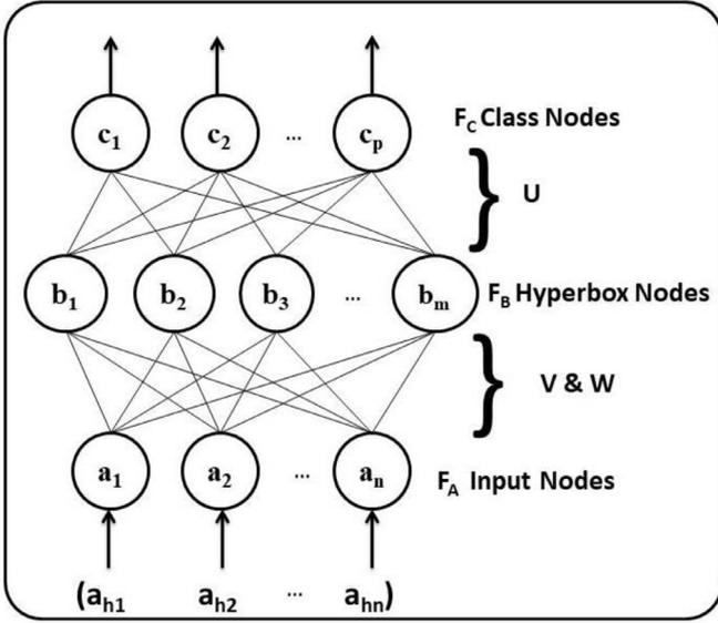
Fig. 2. The structure of FMM.
