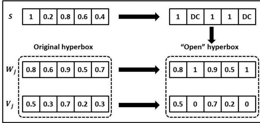
Fig. 5. An example of the generated solution, original hyperbox and “Open” hyperbox. where  $S$  is the generated solution,  $W_j$  and  $V_j$  are the maximum and minimum points of the original hyperbox, respectively. The “Open” hyperbox based on generated solution is shown in the right.
